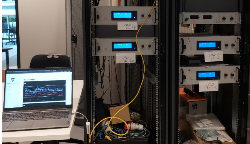
Figure 2: Lab simulation setup showing the 4 Delta Elektronika CPSs and a laptop to run the simulations, connected by ethernet link
